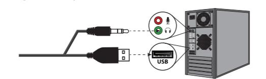
**ATTENTION:** background noise appears if the electrical circuit is poorly shielded on the computer. In this case, connect the USB plug to the USB adapter (not included in the package).
